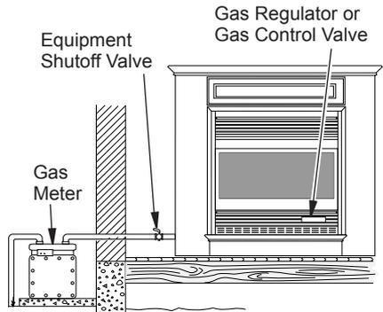
Figure 26 - Checking Gas Joints (Natural Gas Only)
