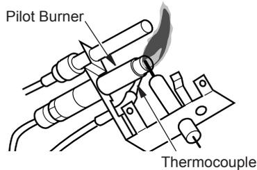
**Figure 47 - Incorrect Pilot Flame Pattern (Propane/LP Remote-Ready Shown)**
