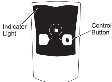
**Figure 43 - On/Off Hand-Held Remote Control Unit**
