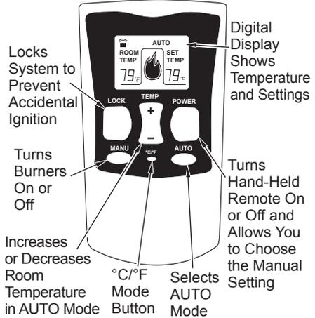
**Figure 44 - Thermostat Hand-Held Remote Control Unit**
