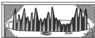
**Figure 49 - Incorrect Burner Flame Pattern**
