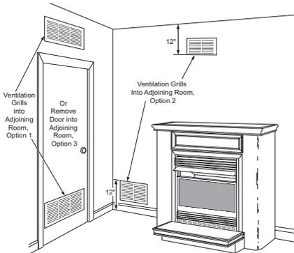
**Figure 4 - Ventilation Air from Inside Building**
