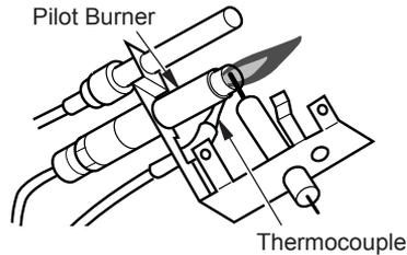
**Figure 46 - Correct Pilot Flame Pattern (Propane/LP Remote-Ready Shown)**
