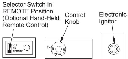
**Figure 42 - Setting the Selector Switch and Control Knob for Hand-Held Remote Operation**
