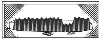
**Figure 48 - Correct Burner Flame Pattern**
