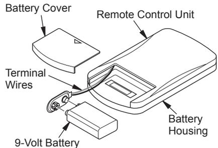
**Figure 30 - Installing Battery in Hand-Held Remote Control Unit**
