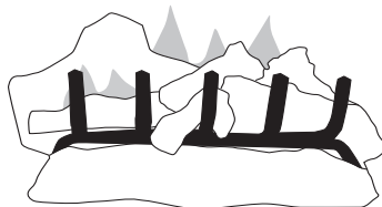
Figure 22 - Correct Burner Flame Pattern
