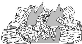
Figure 55 - Typical Flame Pattern
