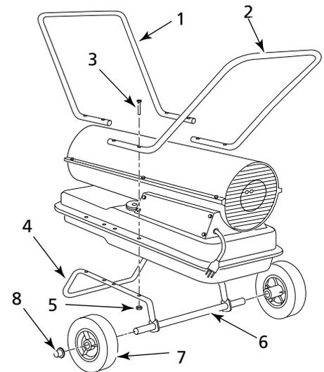
Figure 34 - Handle and Wheel Assembly
