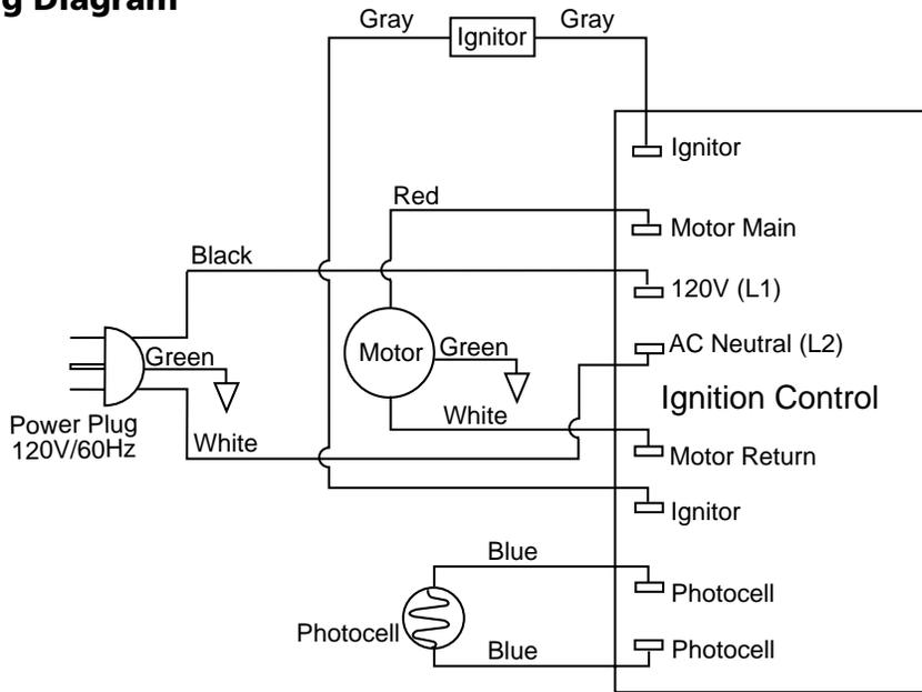
Figure 35 - Wiring Diagram, Models 2E510F and 2E511F
