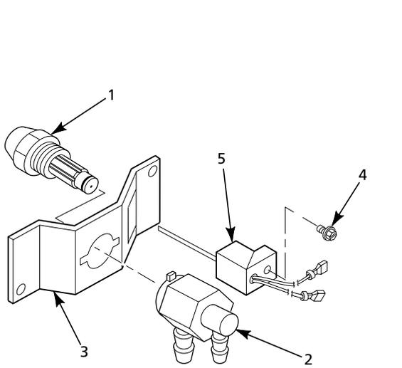
**Figure 29 - Burner Head Assembly for All Models**
