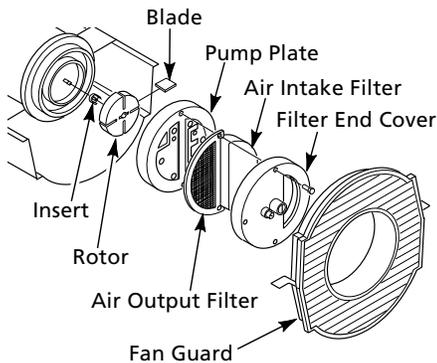
**Figure 23 - Rotor Location, Models 2E510F and 2E511F**
