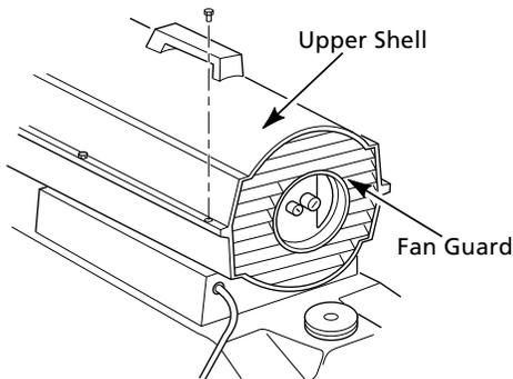
**Figure 7 - Upper Shell Removal, Models 2E510F and 2E511F**
