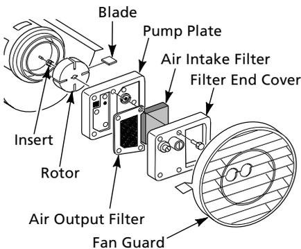
**Figure 24 - Rotor Location, Models 3E218F and 3E219F**
