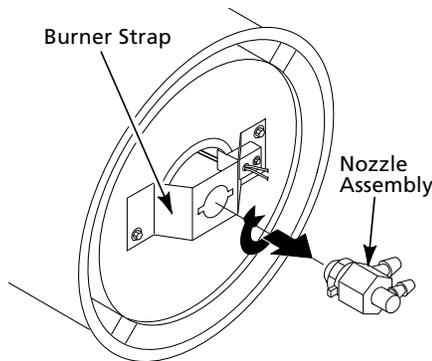
**Figure 20 - Removing Nozzle Assembly, All Models**
