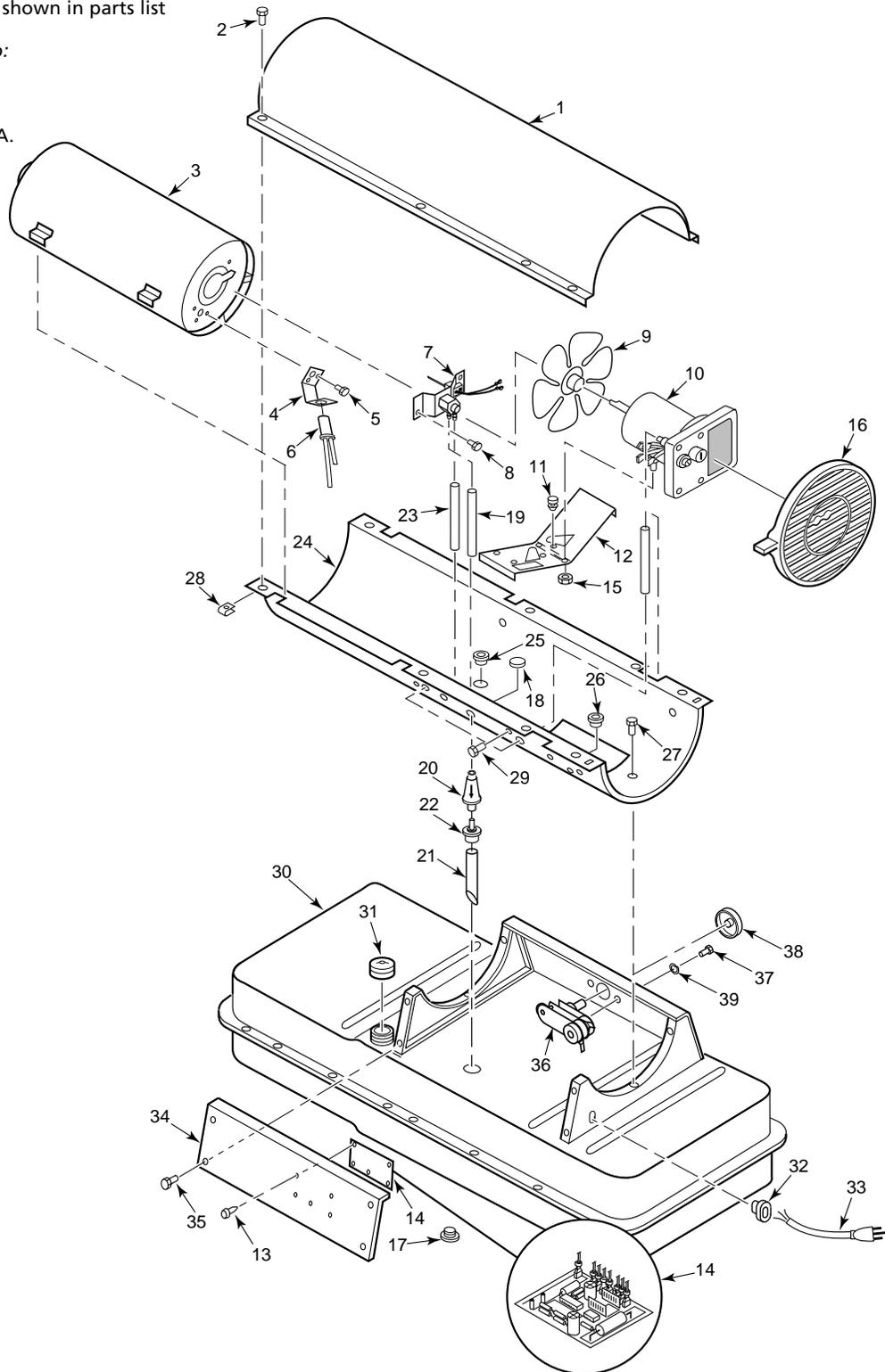
**Figure 33 - Repair Parts Illustration for Model 3E219F**
