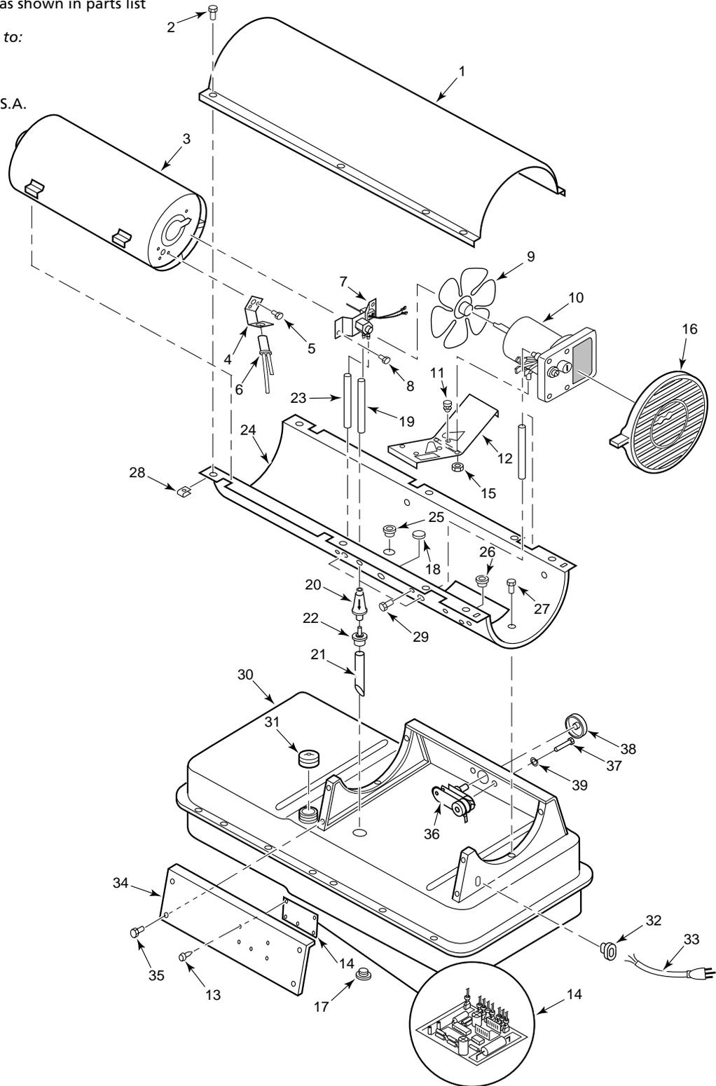
**Figure 32 - Repair Parts Illustration for Model 3E218F**
