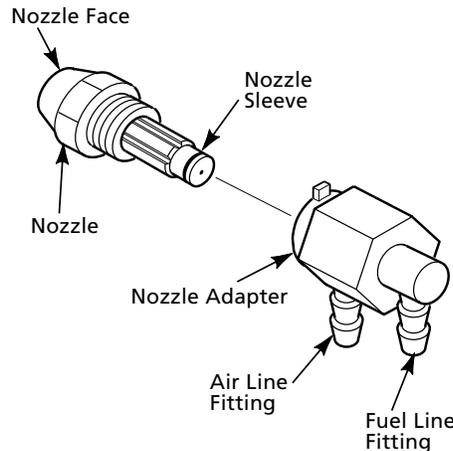
**Figure 21 - Nozzle and Nozzle Adapter, All Models**
