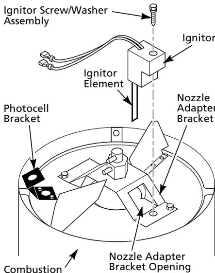
**Figure 17 - Ignitor Replacement**
