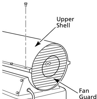
**Figure 8 - Upper Shell Removal, Models 3E218F and 3E219F**
