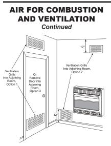
Figure 7 - Ventilation Air from Inside Building
