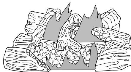
Figure 51 - Typical Flame Pattern
