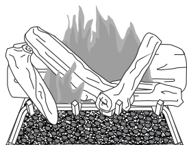
Figure 37 - Typical Flame Pattern
