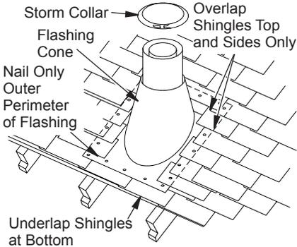
Figure 15 - Flashing Installation
