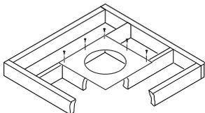
**Figure 13 - Firestop Spacer with Attic Space Above Ceiling**
