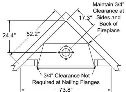
Figure 2 - Corner Installation
