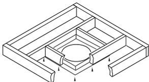
**Figure 12 - Firestop Spacer with Living Space Above Ceiling**
