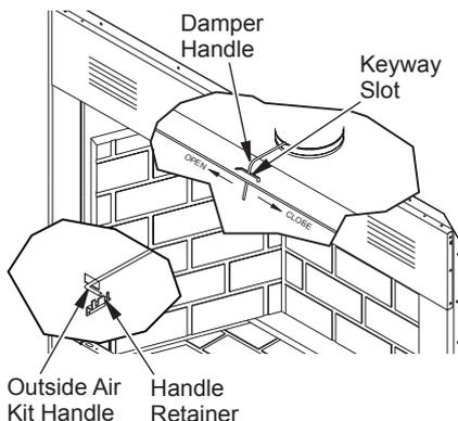
**Figure 24 - Damper and Air Kit Handle**
