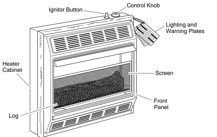
Figure 1 - Vent-Free Gas Log Propane/LP Gas Space Heater
