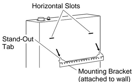
Figure 16 - Mounting Heater Onto Mounting Bracket
