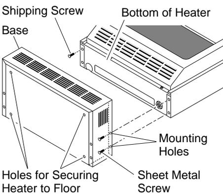
**Figure 18 - Attaching Heater to Hearth Base**
