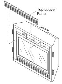
Figure 43 - Removing Top Louver Panel
