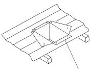
Non-hardening Mastic under all edges of support box before nailing
