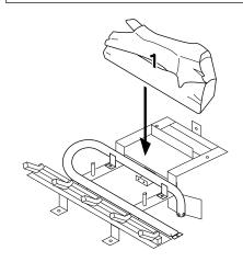
Figure 47 - Installing Log No. 1
