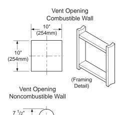
Figure 12 - Vent Opening Requirements
