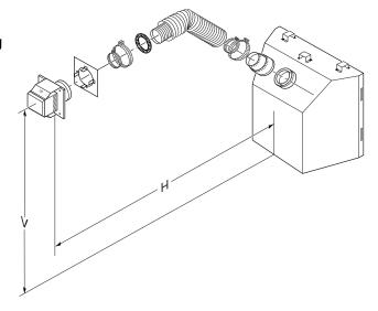
Figure 18 - Horizontal Termination Using Flexible Venting
