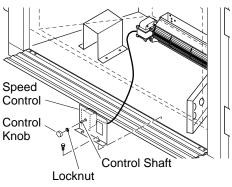
Figure 32 - Attaching Speed Control to Firebox
