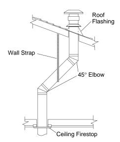
Figure 21 - Offset with Wall Strap and 45° Elbows
