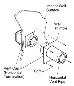
Figure 15 - Connecting Vent Cap with Horizontal Vent Pipe
