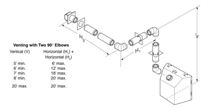
Figure 20 - Horizontal Termination Configuration for Rigid Venting Using Two 90° Elbows with Termination at 90° with Fireplace
