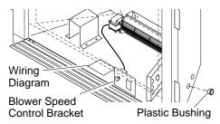
Figure 33 - Installing Plastic Bushing and Wiring Diagram Sticker
