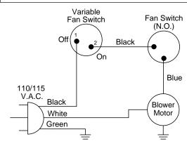
Figure 56 - Blower Wiring Diagram for Thermostat-Controlled Models
