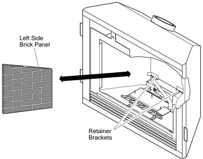
Figure 45 - Installing Left Side Brick Panel
