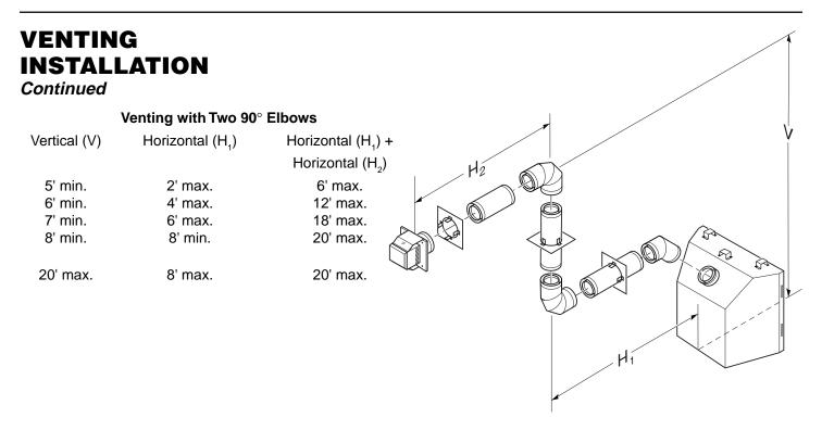
Figure 19 - Horizontal Termination Configuration for Rigid Venting Using Two 90° Elbows
