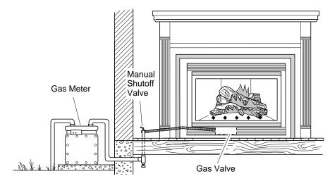
Figure 39 - Checking Gas Joints for Natural Gas Fireplace
