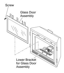
Figure 44-Removing/Replacing Glass Door
