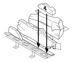
Figure 50 - Installing Log No. 4
