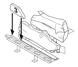
Figure 49 - Installing Log No. 3
