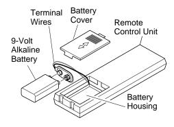
Figure 42 - Installing Alkaline Battery in Hand-Held Remote Control Unit
