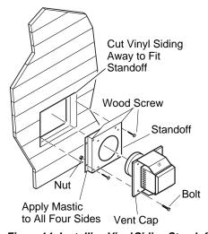
Figure 14 - Installing Vinyl Siding Standoff
