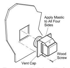
Figure 13 - Installing Horizontal Vent Cap
