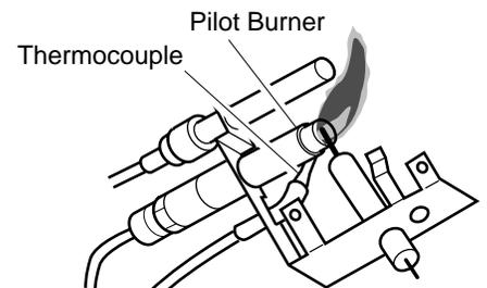
Figure 36 - Incorrect Pilot Flame Pattern
