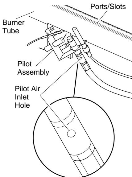
**Figure 38 - Pilot Inlet Air Hole**
