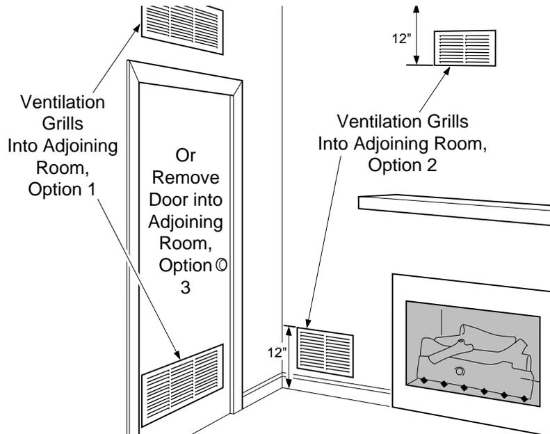
Figure 2 - Ventilation Air from Inside Building
