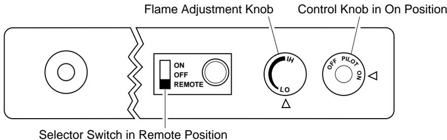
Figure 33 - Setting the Selector Switch, Control Knob, and Flame Adjustment Knob for Remote Operation
