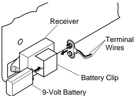
**Figure 20 - Installing Receiver on the Back of the Base**
