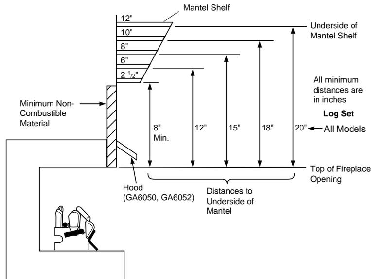
**Figure 7 - Minimum Mantel Clearances When Using Hood**
