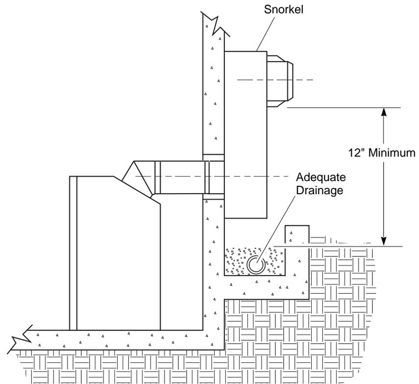
Figure 10 - Snorkel Termination with Drainage Pipe
