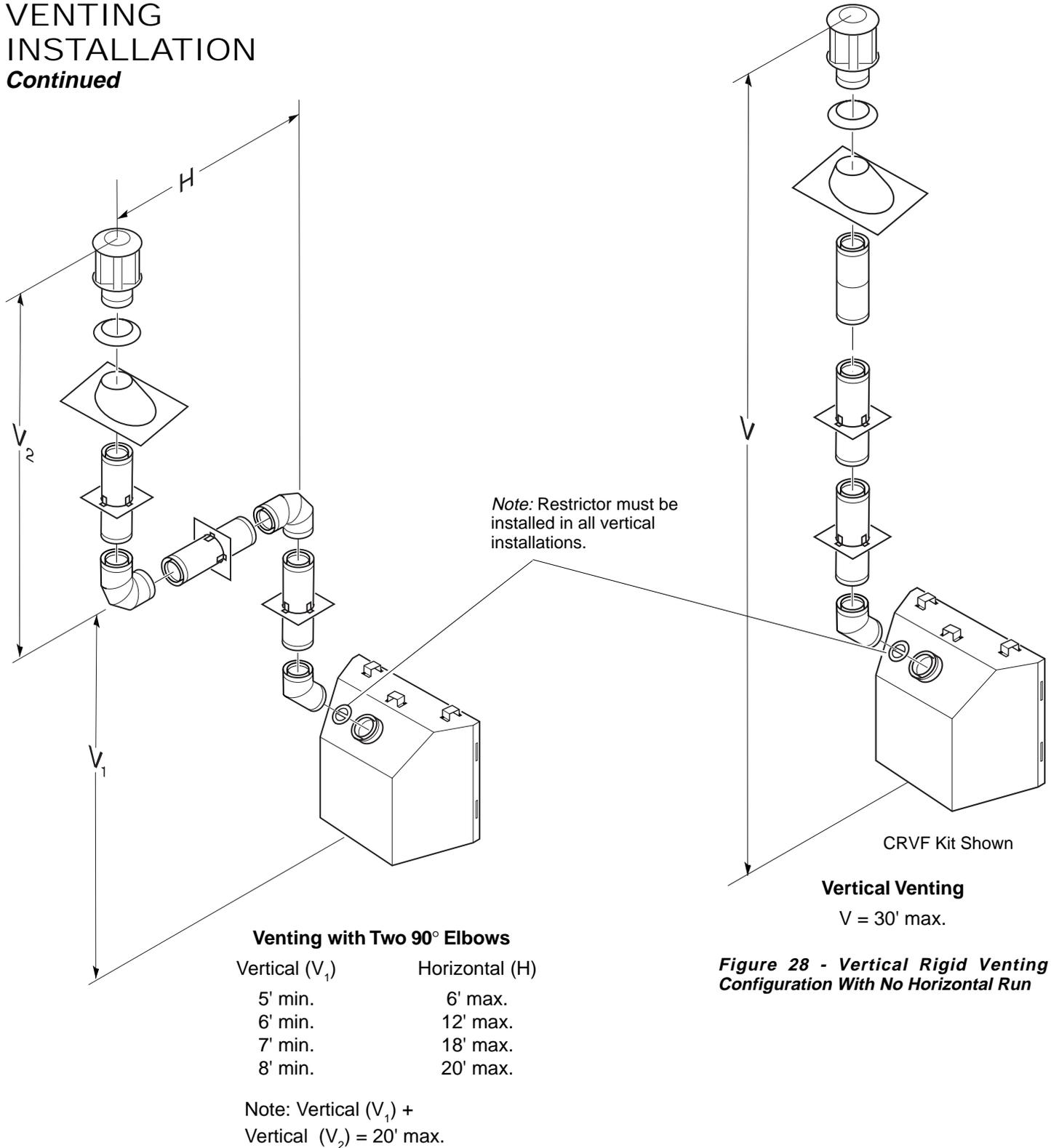
**Figure 27 - Vertical Rigid Venting Configuration Using Two 90° Elbows**
