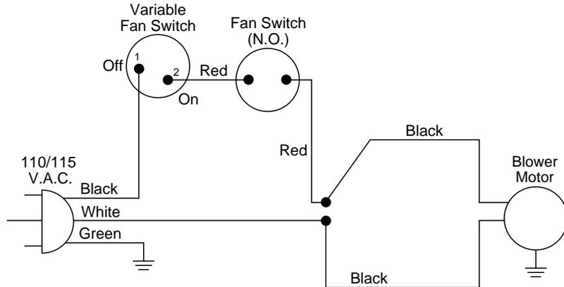
Figure 56 - Blower Wiring Diagram for Thermostat-Controlled Models
