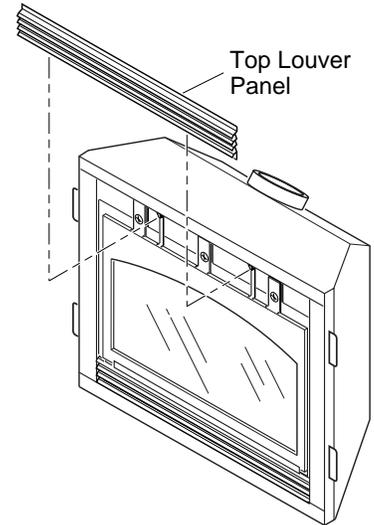
**Figure 43 - Removing Top Louver Panel**
