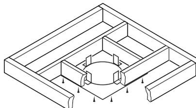
**Figure 22 - Installing Firestop**
