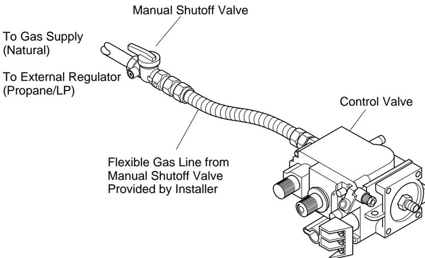
**Figure 36 - Attaching Flexible Gas Line to Control Valve**
