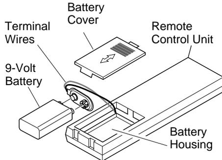
**Figure 42 - Installing Battery in Hand-Held Remote Control Unit**
