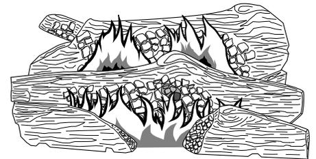
Figure 55 - Typical Flame Pattern for CDV34(N/P)(A).
