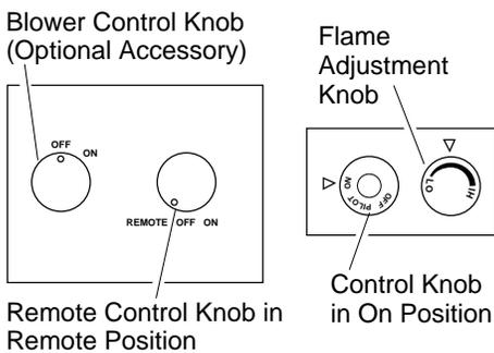
Figure 53 - Setting for Remote Operation
