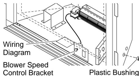
**Figure 33 - Installing Plastic Bushing and Wiring Diagram Sticker**
