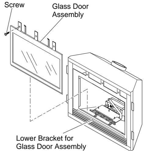
**Figure 44- Removing/Replacing Glass Door**
