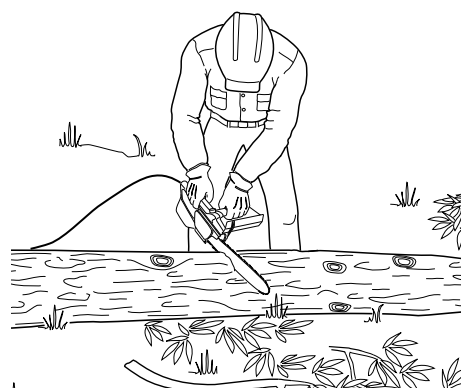
Figure 14 - Bucking Log With Entire Length On Ground
