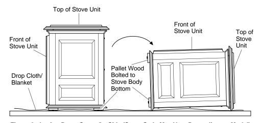
Figure 6 - Laying Down Stove On Side (Stove Style May Vary Depending on Model)
