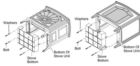
Figure 10 - Attaching Stove Bottom (Amity™ Model Shown)
