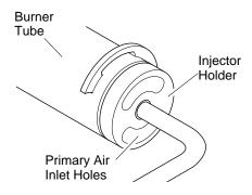
Figure 34 - Injector Holder On Outlet Burner Tube
