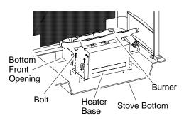
Figure 15 - Placing Heater Base In Stove Cavity (Appearance May Vary Depending on Model)
