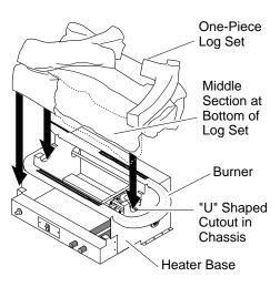
Figure 17 - Installing One-Piece Stove Log Set (Remote-Ready Log Heater Shown)
