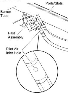
Figure 35 - Pilot Inlet Air Hole
