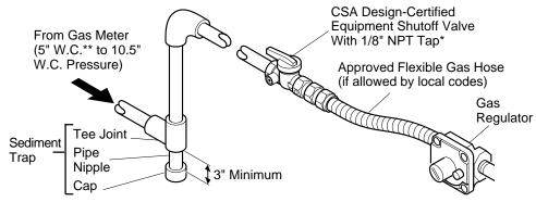
Figure 21 - Gas Connection (SVYD18N and FSVYD18N Series)
