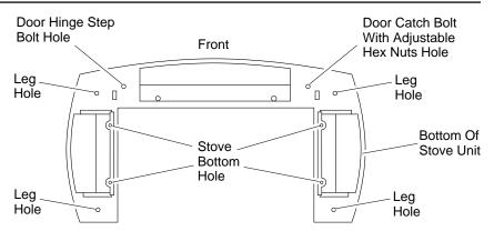
Figure 8 - Locating Threaded Holes for Stove Bottom, Legs, and Door Attachment (Appearance May Vary Depending on Model)
