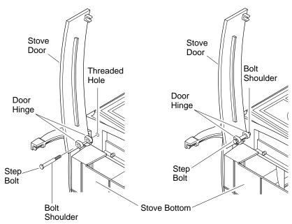
Figure 13 - Attaching Stove Door (Appearance May Vary Depending on Model)
