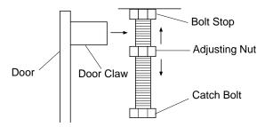
Figure 14 - Catch Bolt and Door Claw Orientation
