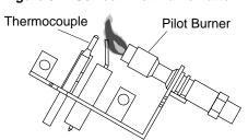
Figure 33 - Incorrect Pilot Flame Pattern
