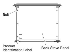
Figure 5 - Removing Back Panel
