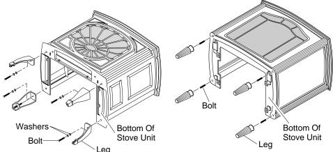
Figure 9 - Attaching Stove Legs (Amity™ Model Shown)
