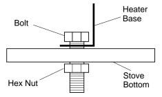
Figure 16 - Fastening Heater Base to Stove Drop Bottom
