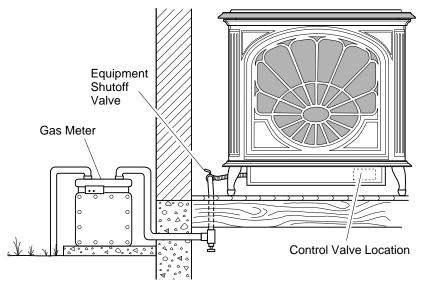
Figure 23 - Checking Gas Joints (Amity™ Stove Model Shown)
