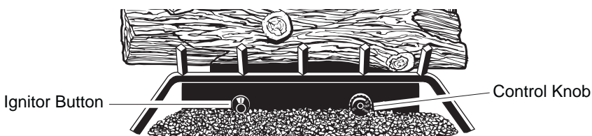
Figure 24 - Control Knob and Ignitor Button Location
