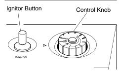
Figure 16 - Control Knob In The OFF Position
