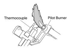
Figure 19 - Incorrect Pilot Flame Pattern
