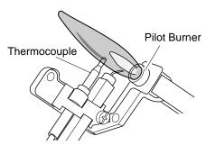
Figure 18 - Correct Pilot Flame Pattern
