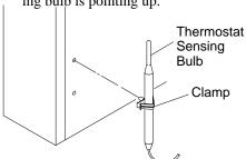
Figure 5 - Attaching Thermostat Sensing Bulb
