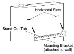
Figure 11 - Mounting Heater Onto Mounting Bracket
