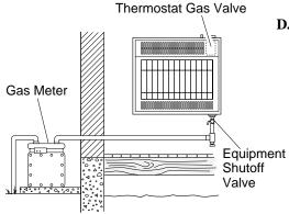
Figure 15 - Checking Gas Joints
