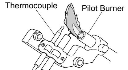
**Figure 30 - Incorrect Pilot Flame Pattern**
