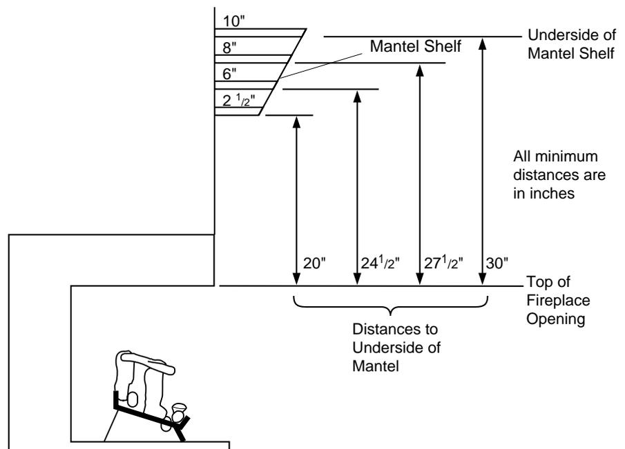
**Figure 15 - Minimum Mantel Clearances for Built-In Installation**
