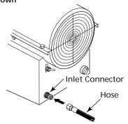
Figure 5 - Hose and Inlet Connector
