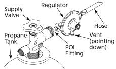
Figure 4 - Regulator With Vent Pointing Down
