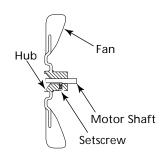
Figure 8 - Fan Cross Section
