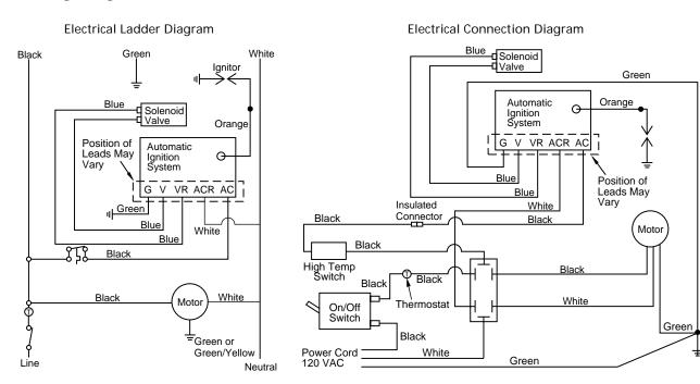
Figure 9 - Electrical Ladder Diagram
