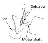
Figure 7 - Fan, Motor Shaft, and Setscrew Location
