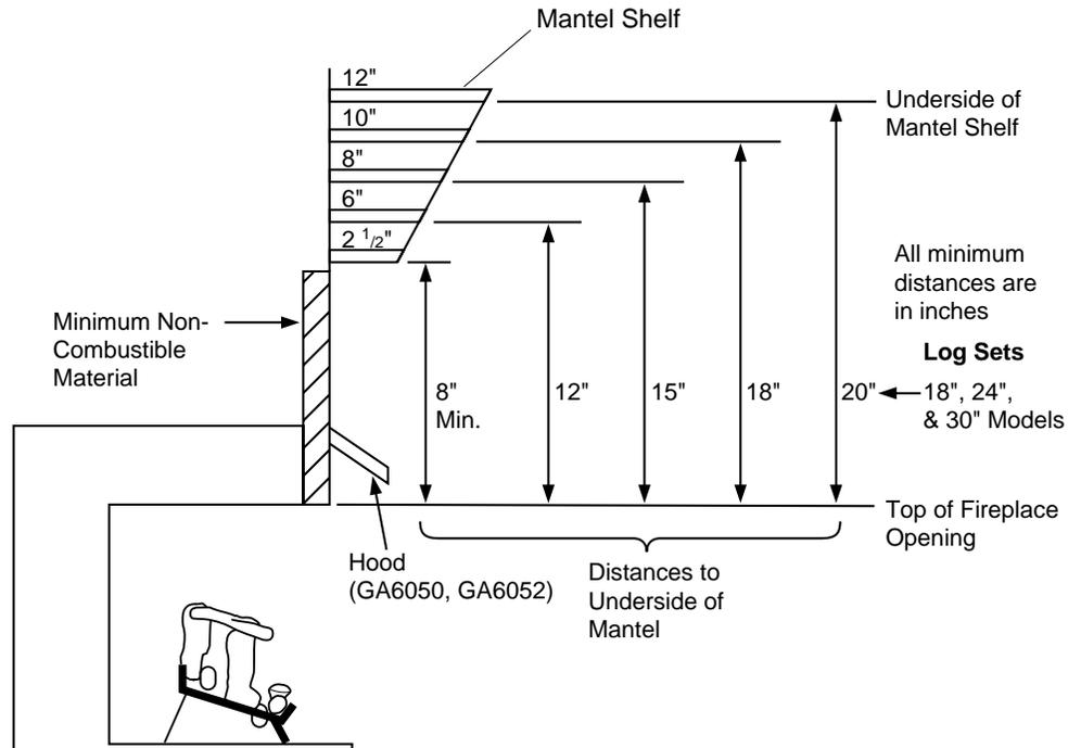
**Figure 8 - Minimum Mantel Clearances When Using Hood**
