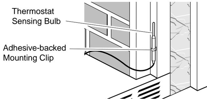
**Figure 39 - Locating Thermostat Sensing Bulb on Factory-built Metal Fireplace**
