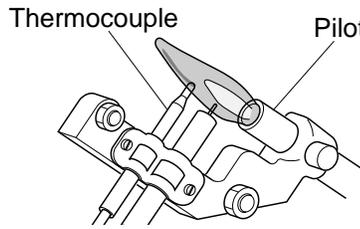
**Figure 31 - Correct Pilot Flame Pattern**
