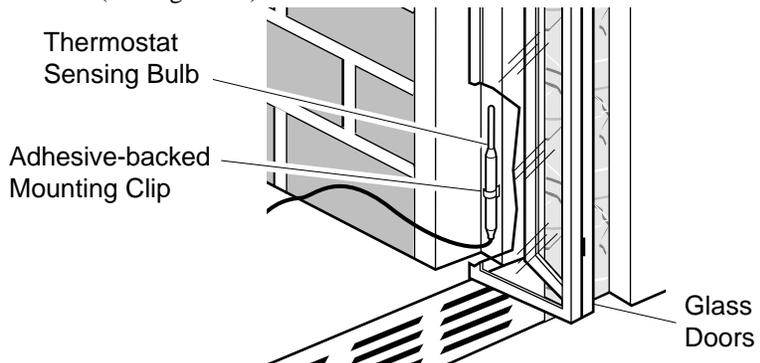
**Figure 40 - Installing Thermostat Sensing Bulb behind Glass Doors**
