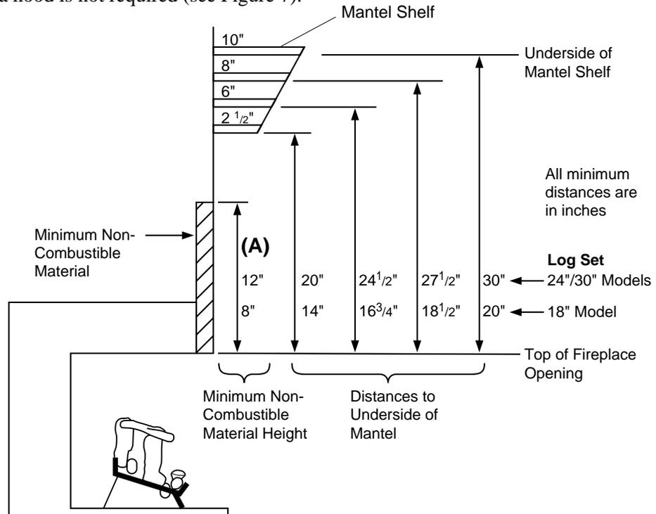
**Figure 7 - Minimum Mantel Clearances Without Using Hood**
