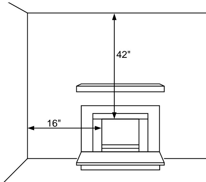
*Figure 5 - Minimum Clearance to Wall and Ceiling*
