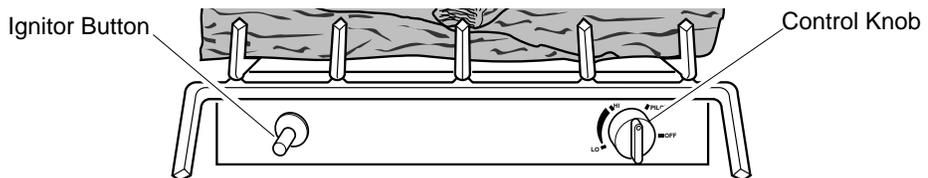
Figure 22 - Control Knob and Ignitor Button Location
