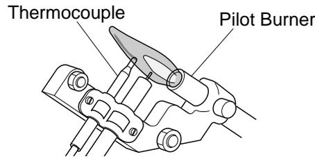
**Figure 24 - Correct Pilot Flame Pattern**
