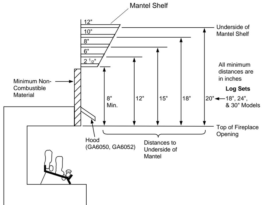
**Figure 7 - Minimum Mantel Clearances When Using Hood**
