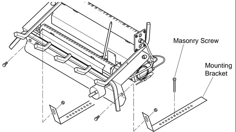
**Figure 12 - Attaching Mounting Brackets to Heater**
