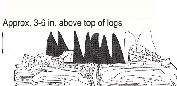
Fig. 18 - Correct Pilot Flame Pattern with Control Knob Set to High Flame (5)
