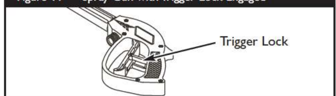
Figure 11 — Spray Gun with Trigger Lock Engaged
