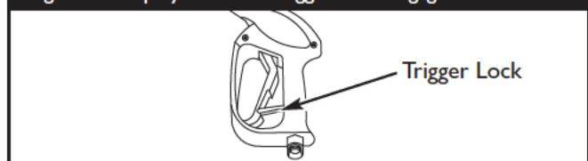
Figure 9 — Spray Gun with Trigger Lock Engaged
